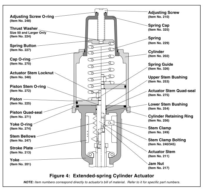
movement into the bore. For *air-to-extend* configurations, repeat this process without the thrust washers or springs. Once the piston is installed and leveled, center the spring on the piston.
