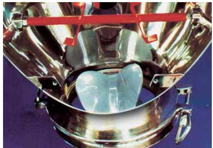
Rotary Valve installed with "bridge-breaker".
