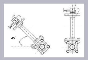
Cryogenic valves are optimally oriented with the stem 90° from the horizontal plane. PBM cryogenic valves are capable of operating with the stem oriented as low as 45° above the horizontal plane.
