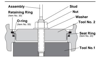
Figure 1: High Temperature Seat Ring (NOTE: Item numbers correspond to the valve's bill of material)
