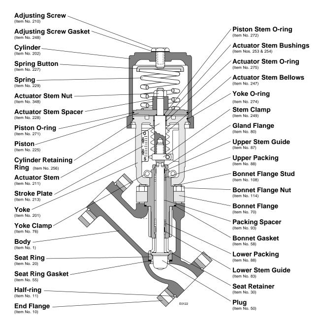
Figure 2: Sectioned View of Standard Mark Eight Control Valve
