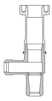
Figure 2: Angle Body Construction
