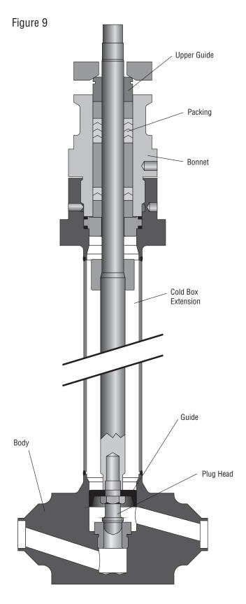
For small, precision flow in cryogenic service, the Mark Six Low Flow is the answer. Using the same principles as the standard Mark Six, the Mark Six Low Flow was redesigned to give precision control over valves with very small capacities. The smallest valve can have a maximum capacity as low as 0.012 C<sub>V</sub>.
