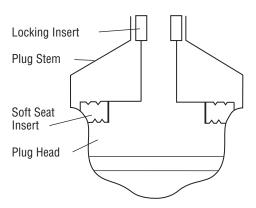
Figure 4: Threaded Plug Head
