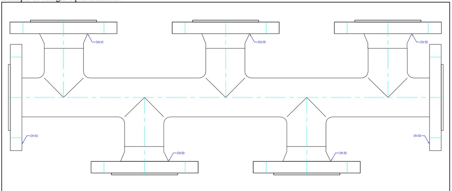
Example of inclined reduced manifold.
