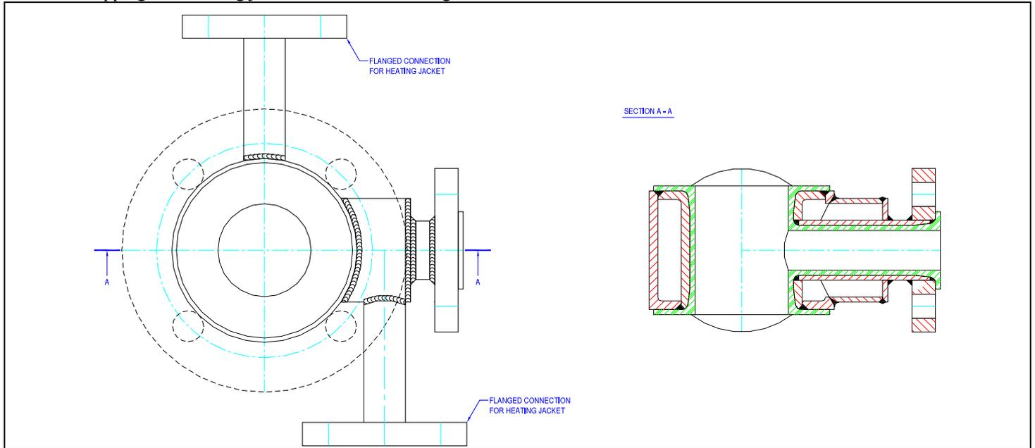
Instrument tapping with heating jacket – version with threaded connections.
