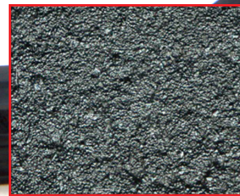
Flowserve fine grain UNCD coated seal face under 1000x magnification
