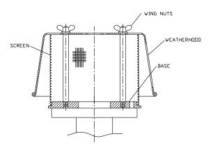
Sizes Available. 2" (DN 50) through 12" (DN 300) aluminum units flanged to mate with 125# ANSI and DIN PN 16 flat face flanges. All other materials mate with 150# ANSI and DIN PN 16 raised face flanges. 16" (DN 400) through 24" (DN600) units flanged to mate with applicable ANSI or API flat face flange connections.
